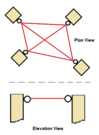
Measurements are to be taken from fixing point to fixing point as shown.
